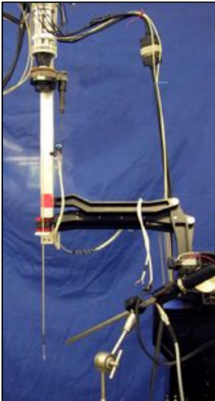
4mm Snake-Like Robot for throat
