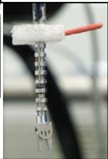
4mm Snake-Like Robot for Throat
