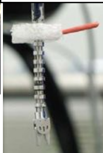
4mm Snake-Like Robot for Throat
