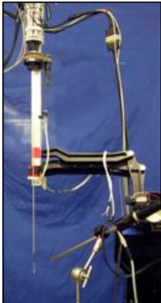
4mm Snake-Like Robot for Throat
