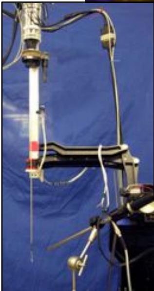
4mm Snake-Like Robot for Throat
