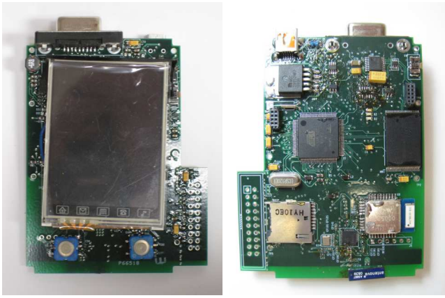
Fig. 1. Picture of the Egs platform. The front side of the Egs platform includes a 2.4 inch LCD and two user buttons (left). The Atmel SAM3U2C microcontroller, TI CC2520 radio, Mitsumi Bluetooth module, 2 Gb NAND flash, and a micro SD card slot is located on the back side of the board (right). The pins that are located next to the micro SD card slot are used for the JTAG and can be detached at the end of the development phase.
