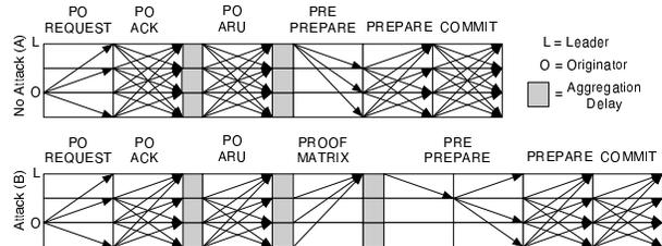
Figure 2: Common case operation of Prime ( $f = 1$ ). Part A shows the messages and protocol rounds when the leader is correct. Part B shows the delay added by a malicious leader that performs well enough to stay in power. The malicious leader ignores PO-ARU messages and sends its PRE-PREPARE to only one correct server.
