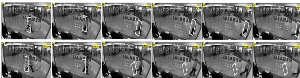
Figure 5: The tracking results of HKSL (row 1) and IPCA (row 2) in Experiment 1 over representative frames (17, 27, 33, 39, 43, and 46) from Video 1 in the scenarios of image distortions and partial occlusions.
