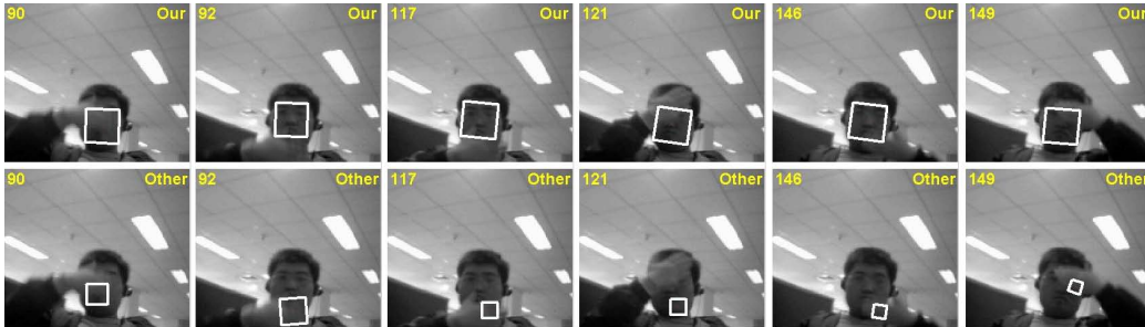
Figure 8: The tracking results of HKSL (row 1) and IPCA (row 2) in Experiment 4 over representative frames (90, 92, 117, 121, 146, and 149) from Video 4 in the scenario of occlusions.
