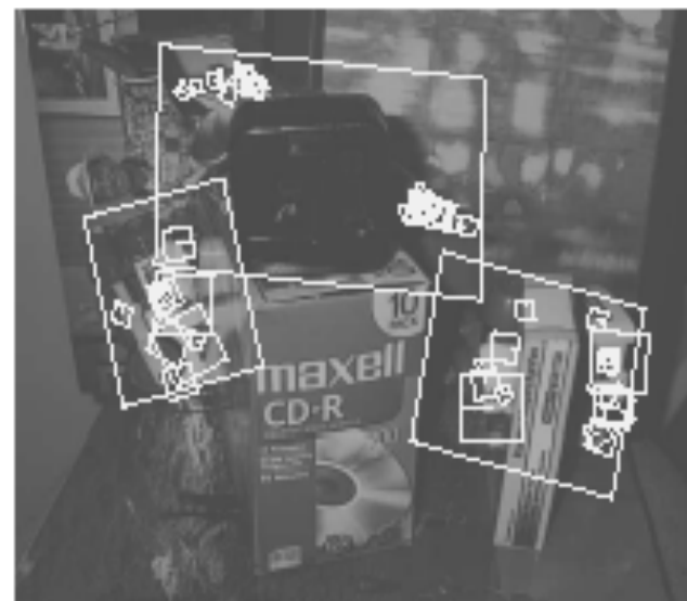
Figure 12: The training images for two objects are shown on the left. These can be recognized in a cluttered image with extensive occlusion, shown in the middle. The results of recognition are shown on the right overlaid on a reduced contrast version of the image. A parallelogram is drawn around each recognized object showing the boundaries of the original training image under the affine transformation solved for during recognition. Smaller squares indicate the keypoints that were used for recognition.
