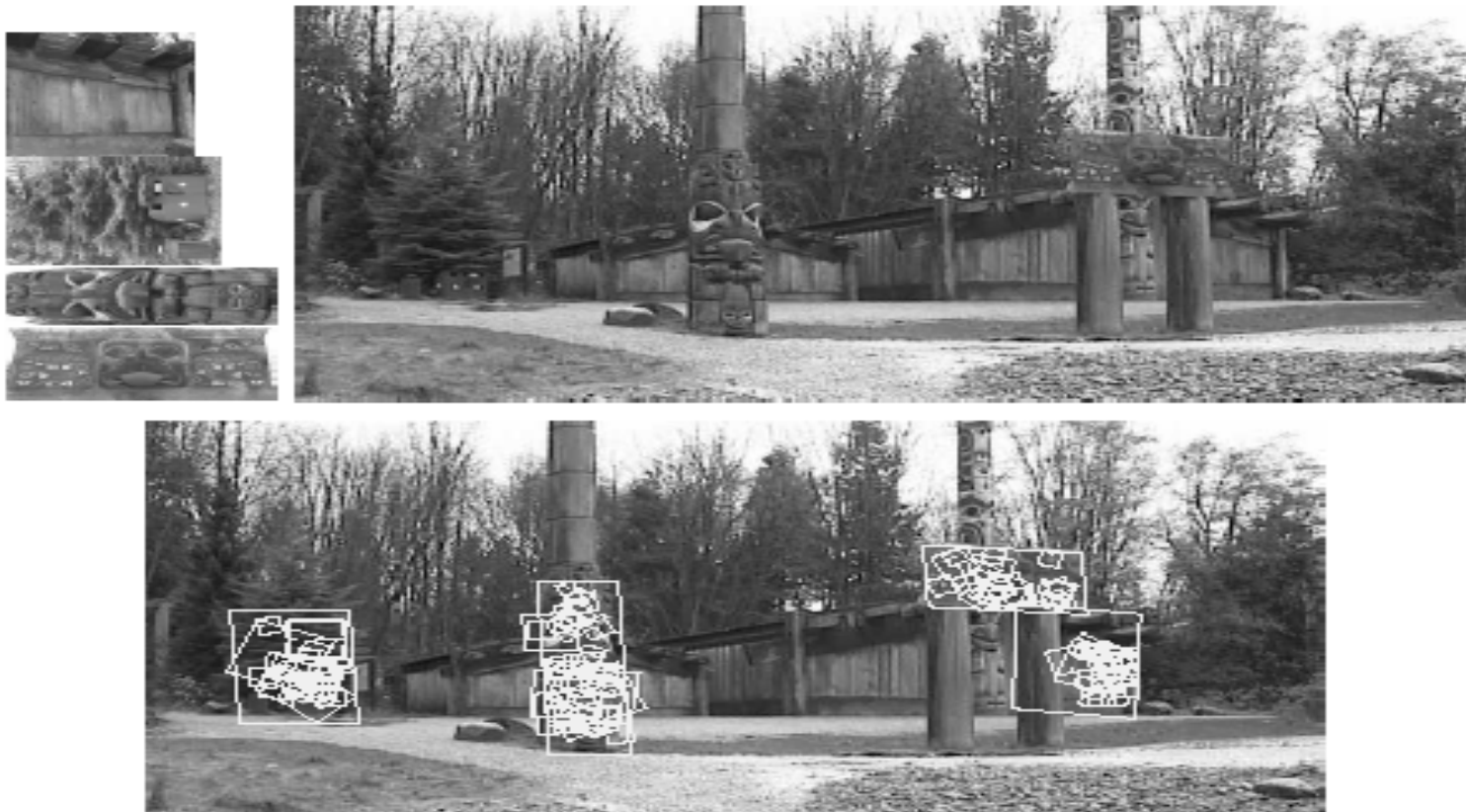
Figure 13: This example shows location recognition within a complex scene. The training images for locations are shown at the upper left and the 640x315 pixel test image taken from a different viewpoint is on the upper right. The recognized regions are shown on the lower image, with key-points shown as squares and an outer parallelogram showing the boundaries of the training images under the affine transform used for recognition.
