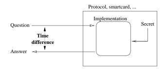
Figure 1: The timing attack principle.
