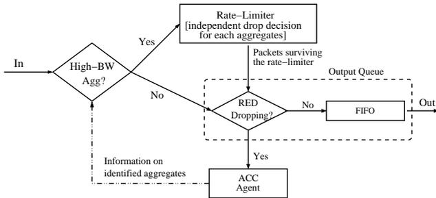
Figure 2: **Architecture of an ACC-enabled router.** Packets of high-bandwidth aggregates pass through the rate-limiter. All packets dropped by RED are passed to the ACC Agent for identifying aggregates.
