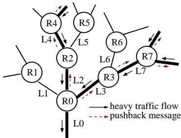
Figure 1: Pushback takes rate-limiting closer to the source(s).
