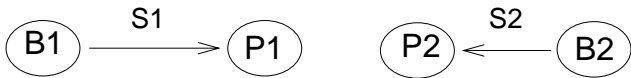
Figure 6: A two cell configuration where both pads are in range of their respective base stations and also in range of each other. The base stations are sending data to their respective pads, and each stream is generating data at a rate of 64 packets per second and using UDP for transport.
