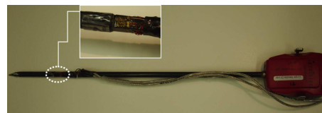
Fig. 3. Modified da Vinci instruments with strain gages in a Wheatstone full bridge configuration. Inset picture: Close-up of the strain gage and wiring.
