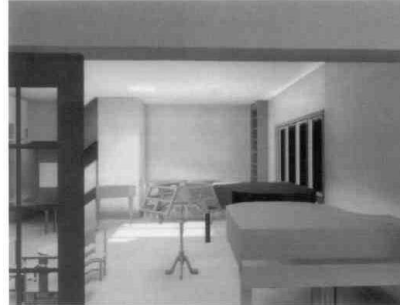
Plate 3: A particularly bad reference frame produced by our test-bed. Some areas of the image near the door were occluded in both reference frames, mostly because of prediction error.
