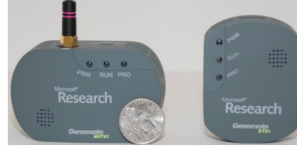
Figure 2: Two types of Genomotes designed for RACNet. The wireless node (on the left) controls several wired nodes (on the right) to reduce the number of wireless sensors within the same broadcast domain.
