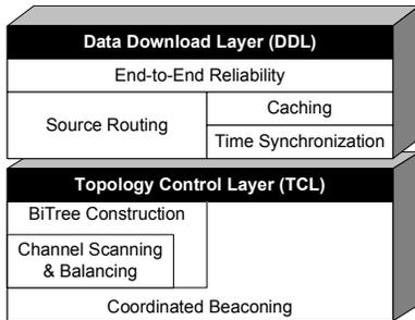
Figure 1: Reliable Data Collection Protocol (rDCP) architecture. The Topology Control Layer (TCL) maintains the tree topology while the Data Download Layer (DDL) reliably downloads data from individual master nodes.
