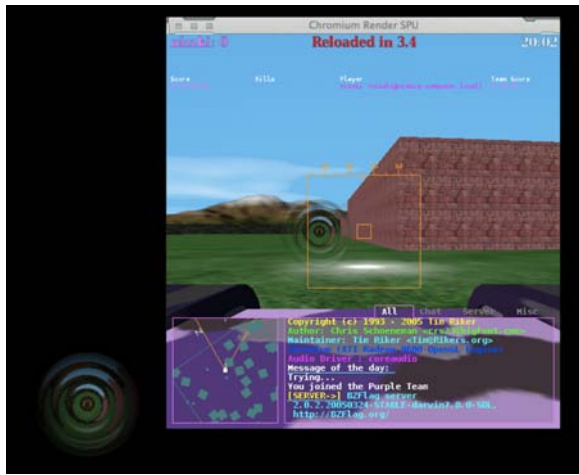
Figure 5: Extracting a single missile object from the BZFlag application. BZFlag issues between 300 and 1000 drawing blocks per frame, depending on the viewing parameters, number of missiles, and other game state. The ability for WHEN statements to use the application’s namespace (in this case, the stack) is essential for this sort of application.
