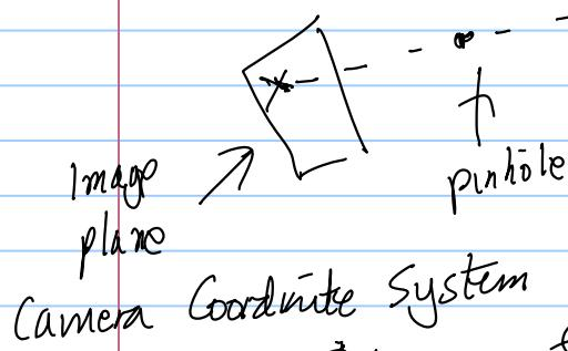
A point in space is projected by a light ray (straight line) which goes through the pinhole and is stopped when it hits the image plane.
