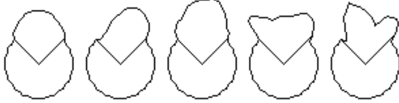
Figure 8 The shape on the left is the mean and the four shapes to its right are the first 4 eigenvectors (plus the mean) of the covariance matrix sorted in the decreasing order of their corresponding eigenvalues.
