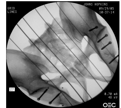
Example C-arm images showing distortion, straight metal wires appear curved due to distortion
