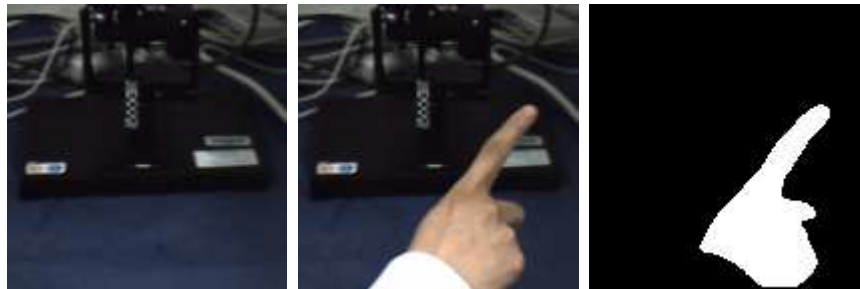
Fig. 2. An example of background image (left), foreground image (middle) and segmentation result (right).
