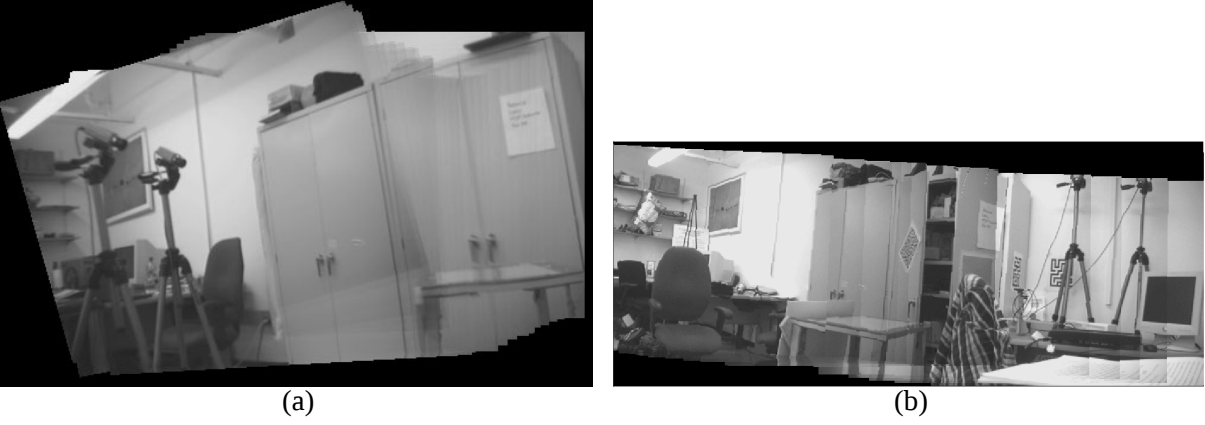
Figure 6: Image mosaicing result for 3D scene image sequence of a laboratory environment with different warping models. (a) Perspective warping (b) Quadratic warping
