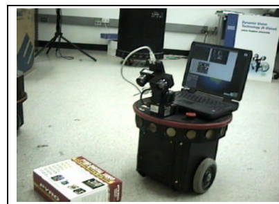
Figure 1: Small mobile robot Speedy equipped with a binocular stereo system.
