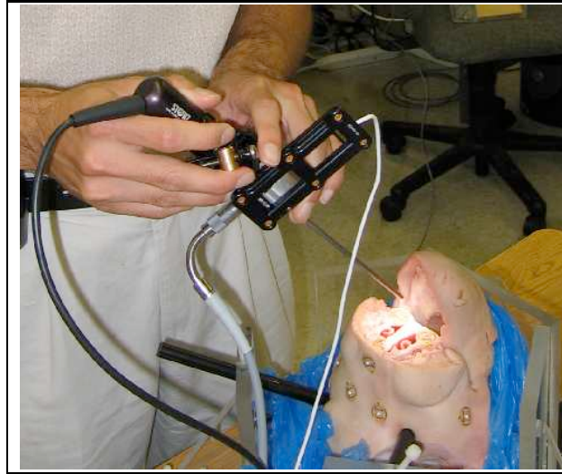
Figure 7. Validation of the approach on a head of a pig cadaver with anatomical structures similar to the human sinuses. OptoTrak data is used as a ground truth to validate the motion estimation of our algorithm.
