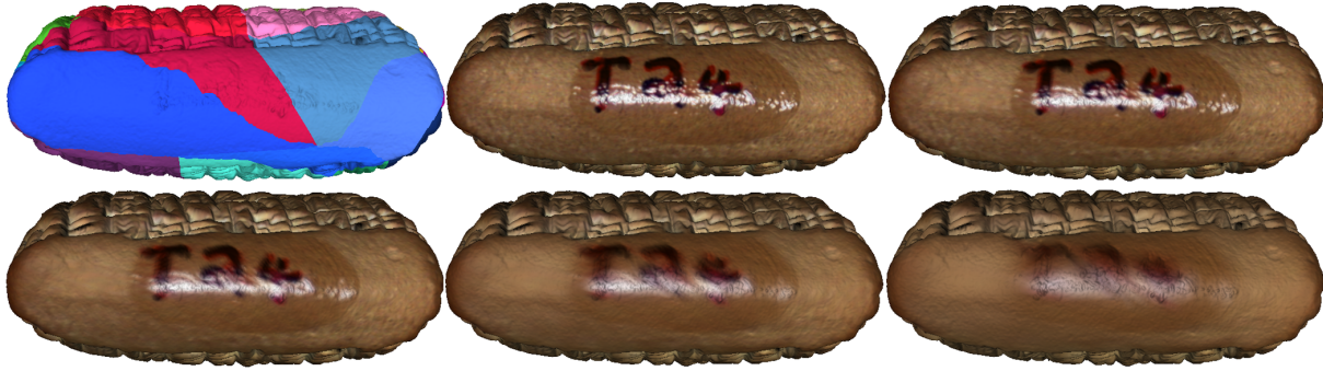
Figure 20: One-million-triangle Cuneiform tablet model, rendered at several of its individual mip-map levels to illustrate the seamless filtering.
