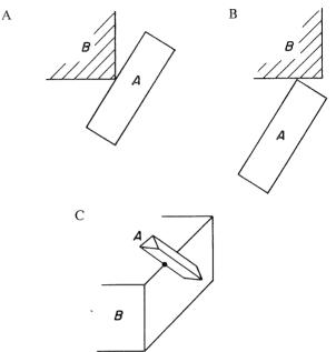
feasible contacts between vertices, edges, and faces of A and B (see Fig. 13) (Lozano-Pérez 1983). Therefore, each face of a C-space obstacle represents a particular type of geometric constraint on A. A range of positions (and orientations) of A can be represented as a volume in the C-space of A, and a motion of A is a curve in the C-space.
