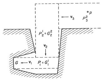
reduces assembly problems for solids into problems involving a point and surfaces in a higher-dimensional space.
