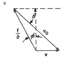
Consider an object controlled by a generalized damper with  $\mathbf{v}_0$  (at an angle  $\theta$  below horizontal) on a rigid surface whose normal points are along the y axis (see Fig. 19A). When the object strikes the surface, the objection can (1) slide to the right, (2) slide to the left, (3) remain motionless. We can use Coulomb's law to determine which of these three possibilities will occur.
