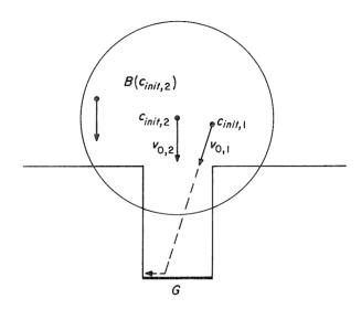
configuration and velocity at time t, for initial position  $c_{init,i}$  and nominal velocity  $v_{0,i}$ .
