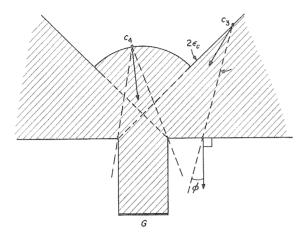
by testing whether all possible predicted trajectories have attained the goal. This satisfies the requirements of the formalism because of the way control error is modeled—we have assumed that the control error is constant during a trajectory. A more realistic model of error would yield more robust predicates, combining position, velocity, and time information to detect presence at the goal.
