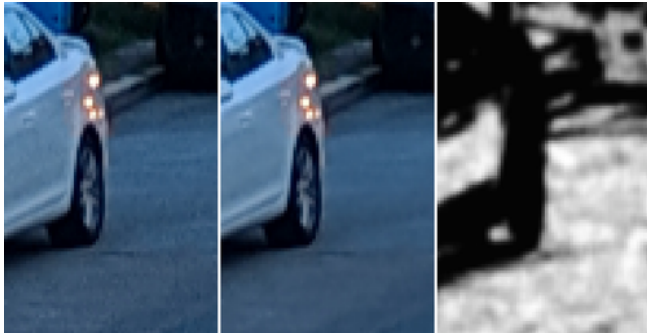
Fig. 24. Denoising: Example effect of local kernel denoising, Left: Low light image without local kernel denoising, k_{denoise} = 1.0 . Middle: image with strong local kernel denoising k_{denoise} = 5.0 . Right: local denoising mask. Black pixels denote areas where we do not apply any spatial denoising and adjust kernel values for super-resolution, while white pixels denote areas where we do not observe enough image details to justify super-resolution and adjust the kernel values for denoising. By analyzing the local structure, our algorithm can cover a continuous balance between resolution enhancement and spatio-temporal denoising.
