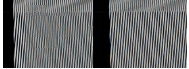
Fig. 27. High frequency artifacts caused by the aperture problem: Left: a high resolution and high frequency test chart image without the rejection logic described in Section S.3. Notice the numerous blocky artifacts visible when zoomed-in. Right: the same image with the rejection logic detecting variance loss showing no fusion artifacts, but some aliasing and color fringing.
