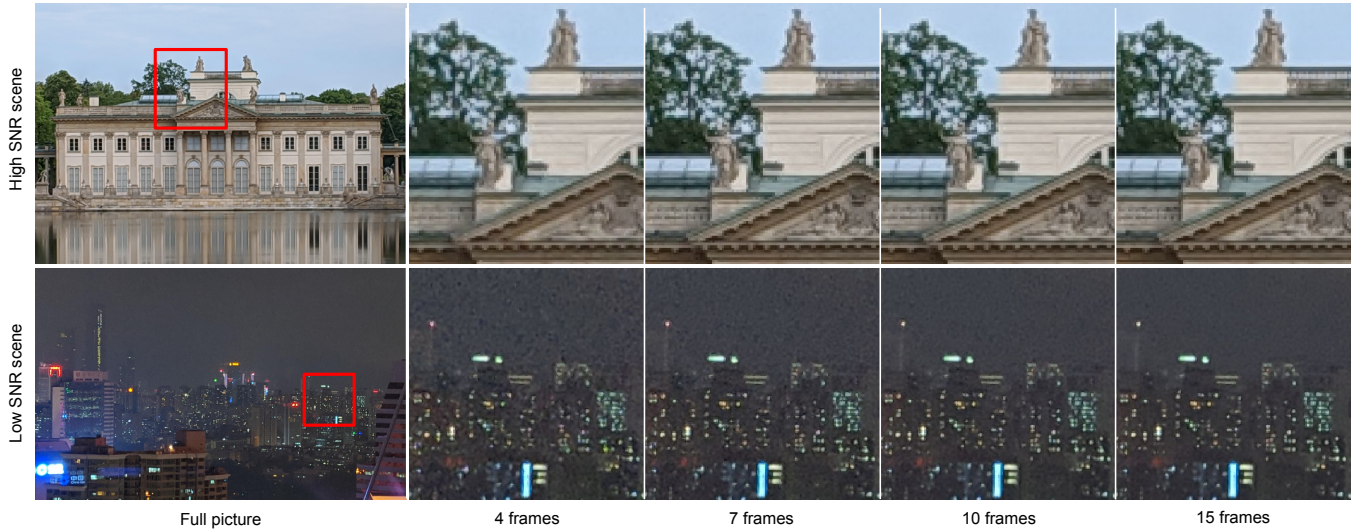
Fig. 19. Visual differences caused by merging a different number of frames in the case of high ( top ) and low ( bottom ) SNR scenes. In the case of the high SNR scenes, we do not observe any image quality increase when using more than seven frames. On the other hand, in the case of low light scenes with worse SNR, we can observe a quality increase and better denoising.
