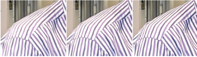
Fig. 12. Left: Merged photograph of a moving person without any robustness. Misalignment causes fusion artifacts. Middle: Merged image with statistical robustness only, some artifacts are still present (we advise the reader to zoom in). Right: Final merged image with both statistical robustness and motion prior. Inclusion of both motion robustness terms helps to avoid fusion artifacts.
