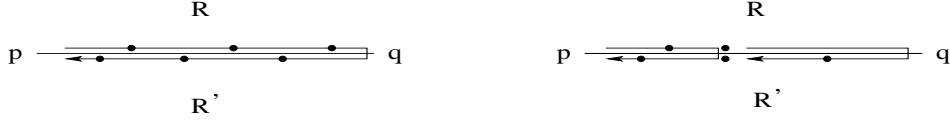
FIG. 5 A loop of vertices (shown as black dots) introduced in the remeshing stage (left). A situation where it has to be broken into two loops (right).
