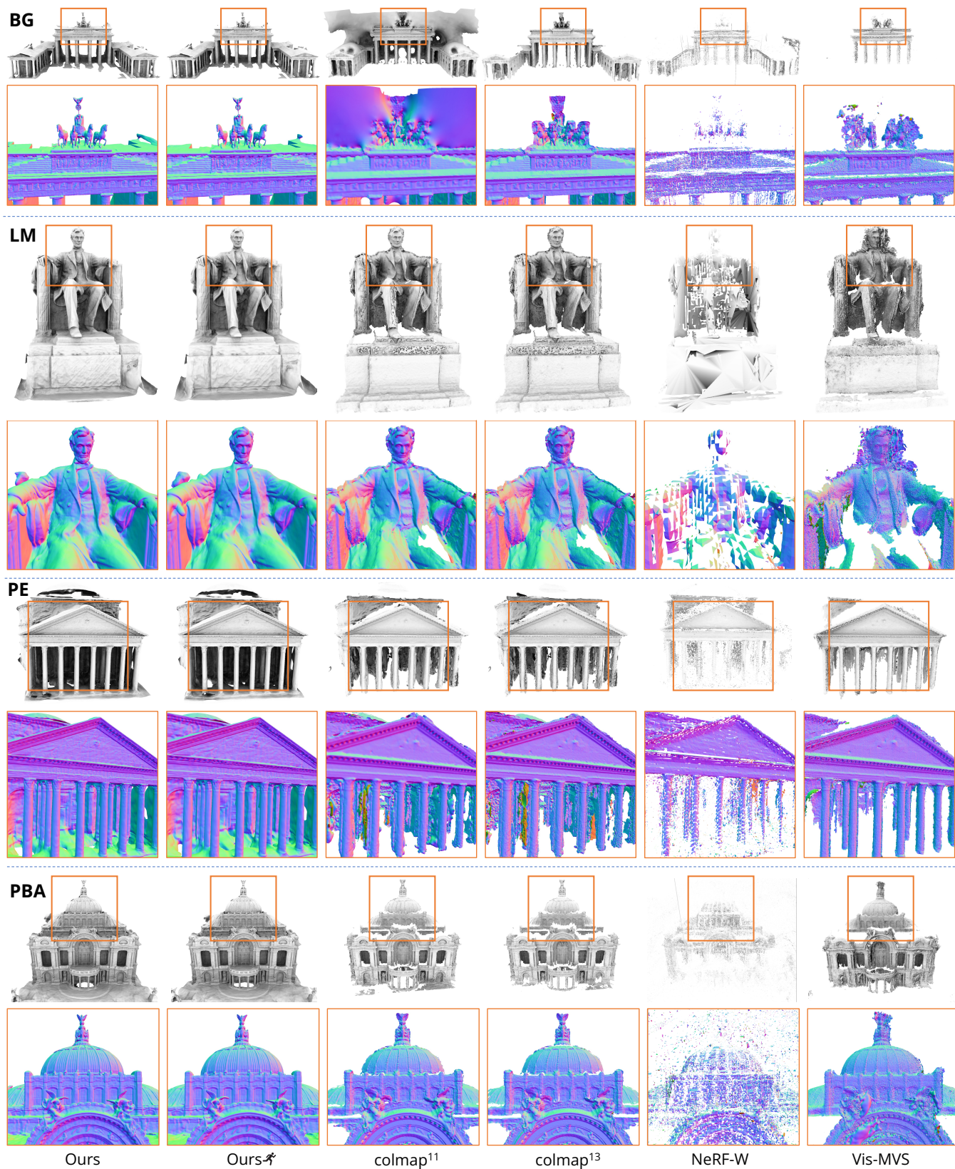
Figure 7: Qualitative results on the Heritage-Recon dataset. As illustrated in the full rendered meshes and the zoomed-in selected regions (in orange), our models yield more complete and higher quality meshes. Zoom in for details. Interactive visualizations can be found at the project page.
