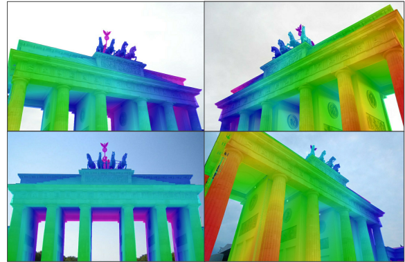
Figure 4: Alignment quality of the LiDAR scan on Brandenburg Gate. We render the LiDAR-scanned point clouds as depth maps by projecting the points to a set of camera views in the aligned SfM coordinate frame. The rendered depth maps are color-coded by depth (warmer colors are closer) and overlaid with the corresponding images. The accuracy of the alignment can be observed in, for instance, the agreement of image and depth edges.
