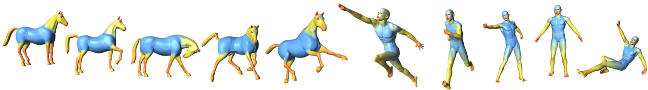
Fig. 2 The shape diameter-function remains largely consistent through pose differences of the same object.
