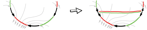
Fig. 7. Splitting the main stream face (left) by our rule produces a simple stream face and removes a pair of in-list/out-list of the main stream face border.
