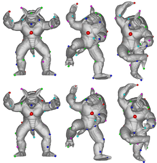
Fig. 10 Correspondence between different poses using the standard (first row) and the equi-affine (second row) metrics. It is clear that the equi-affine metric performs better than the Euclidean one in the presence of bendings. See for example the enlarged red ball in the center of the body that represents a corresponding point mapped from the original surface. (Color figure online)
