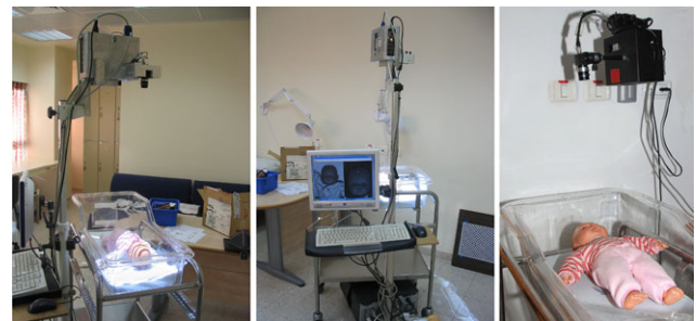
Fig. 13 Structured light scanner used to capture the facial geometry of newborns in the hospital
