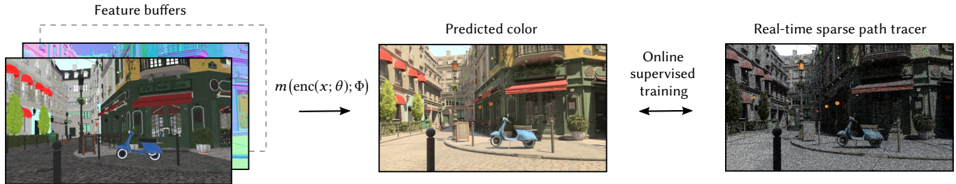
Fig. 8. Summary of the neural radiance caching application [Müller et al. 2021]. The MLP m(\text{enc}(x; \theta); \Phi) is tasked with predicting photorealistically lit pixel colors from feature buffers independently for each pixel . The feature buffers contain, among other variables, the world-space position x , which we propose to encode with our method. Neural radiance caching is a particularly challenging application, because it is supervised online during real-time rendering . The training data are a sparse set of light paths that are continually spawned from the camera view. As such, the neural network and encoding do not learn a general mapping from features to color, but rather they continually overfit to the current environment’s shape and lighting. To support animated content, training has a budget of only one millisecond per frame .
