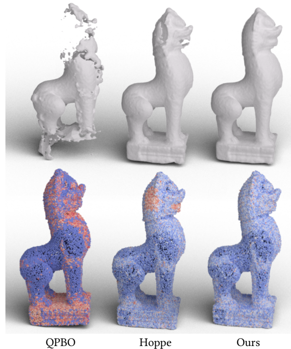
Fig. 17. Normal orientation estimation and corresponding reconstruction results on a large (700k) scanned point cloud.
