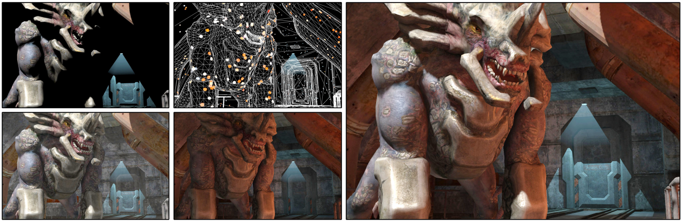
Figure 13: ISPM applied to the NS2 scene. Left top : direct illumination only. Left bottom : direct plus constant “ambient” term. Middle top : photons drawn as large spots on wireframe to illustrate the sampling and geometry. Middle bottom : ISPM’s 3-bounce indirect illumination radiance estimate. Right : composite direct+indirect image rendered by ISPM; compare to the direct+ambient on the lower left. The potentially visible portion of the scene (Figure 9, Cargo Bay only) contains 58k polys on static objects and 15k on dynamic ones, and 4 lights that emit 20k photons total. We import all assets directly from games. This view renders at 21.4 Hz at 1920×1080.
