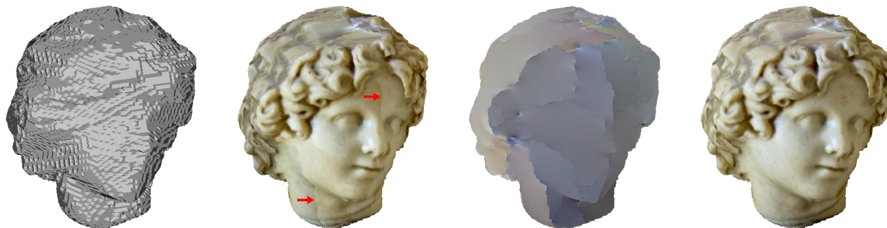
Figure 5. Seam levelling for fragments mosaicing. From left to right: the geometric model, the model with MRF-mosaiced texture (arrows point to residual seams), computed levelling function (contrast enhanced), the model with the seam-levelled texture. Seam levelling successfully removed seams preserving the original detailization.
