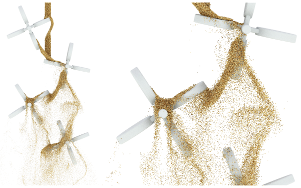
Fig. 14. A vertical Drucker-Prager plastic sand flow is two-way coupled with four rigid paddles, revealing intricate dynamics and flow patterns.
