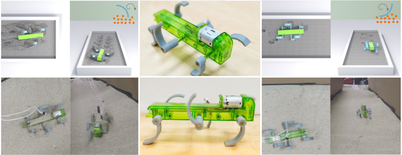
Fig. 16. Our rigid-MPM coupling allows us to simulate terradynamics to predict legged robot’s locomotion on granular media. We 3D print the model from [Li et al. 2013], equip it with motors, and demonstrate how our simulation results (top) match real world footage (bottom) on different motion patterns.
