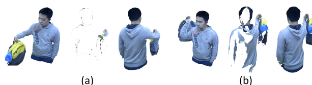
Fig. 17. Comparison of the results of back reconstruction with partially reconstructed results for the backpack sequence. (a) and (b) show comparisons of back-reconstructed results with our partially fused results at frame 160 and frame 490, respectively. The left and middle figures in each group show the partially reconstructed models produced by our algorithm in the first pass rendered from the original camera view and a virtual view, respectively. The right figure in each group shows the back-reconstructed model produced from the final motion field generated in the first pass as rendered from the same virtual view.
