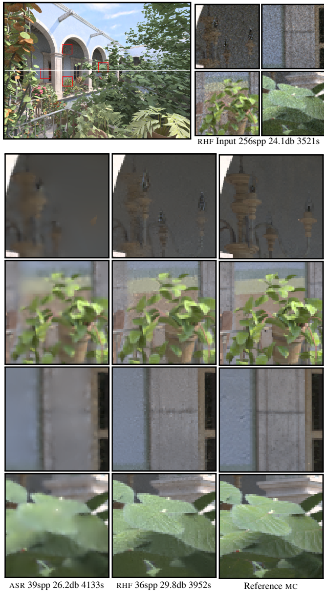
Fig. 10. Comparison of ASR and the proposed method for the san miguel scene. The original 1357 \times 986 Monte Carlo image was rendered with 256 spp. The PSNR values are given for the whole image. This image presents a very complex fine geometry and complex corridors where it is very difficult to capture all the details with few samples. Nonetheless, the proposed algorithm produces acceptable quality and PSNR. The reference image was generated with 65536 samples per pixel. For RHF, the indicated time is the the total time rendering + filtering .
