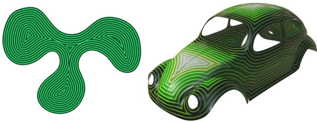
Figure 15: Distance to the boundary on a region in the plane (left) or a surface in \mathbb{R}^3 is achieved by simply placing heat along the boundary curve. Note good recovery of the cut locus, i.e., points with more than one closest point on the boundary.
