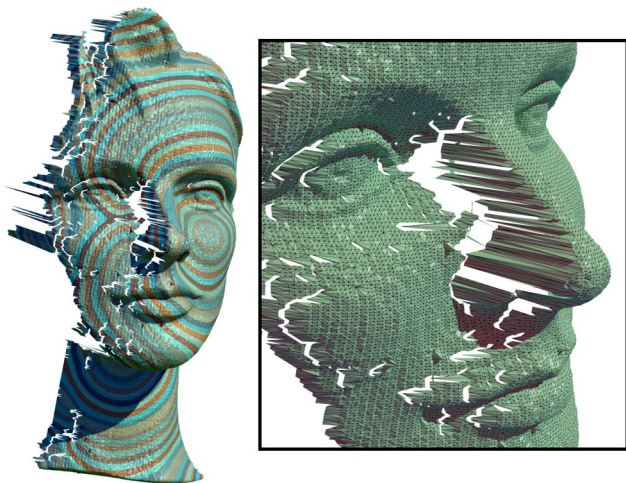
Figure 16: Smoothed geodesic distance on an extremely poor triangulation with significant noise – note that small holes are essentially ignored. Also note good approximation of distance even along thin slivers in the nose.
