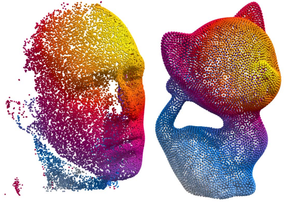
Figure 6: The heat method can also be applied directly to scattered point clouds that lack connectivity information (yellow points are close to the source). Left: face scan with holes and noise; disconnected components receive a constant value (red) Right: kitten surface from Figure 10 with connectivity removed (for reference).
