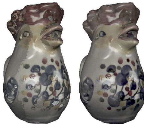
Figure 1: Reconstructing colored surfaces from 3D scans: The texture obtained by pulling color values from the closest scans is shown on the left, while taking color gradients from the closest scans and solving the Poisson equation gives the seamless result on the right.
