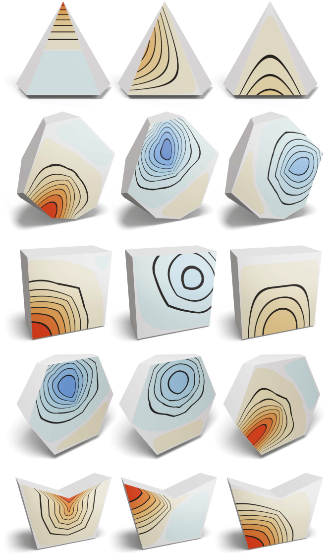
Fig. 8. Cross-sections showing our quadratic shape functions, for different polyhedra: While the shape functions are optimized for smoothness, they may exhibit small gradient discontinuities across virtual faces, visible as sharp corners along iso-curves. For tetrahedra (top), where we reproduce quadratic Lagrange shape functions, the functions are C^1 inside the simplex.
