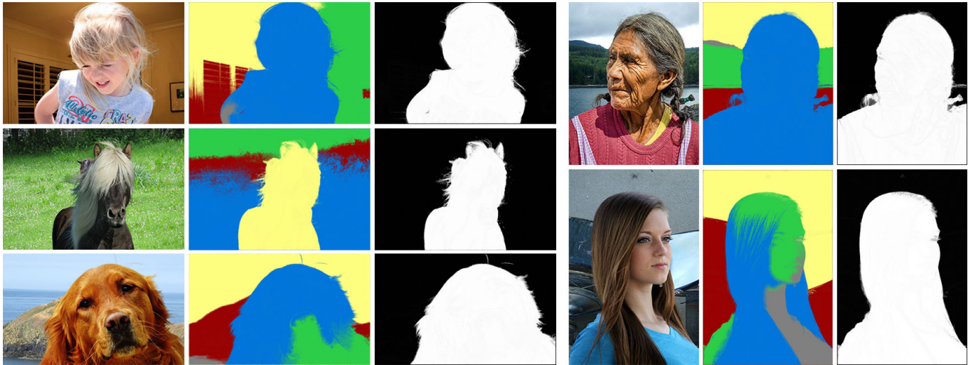
Fig. 12. Our soft segments and the corresponding mattes for the foreground objects. Note that trimaps usually provided for natural matting were not used to produce these results.
