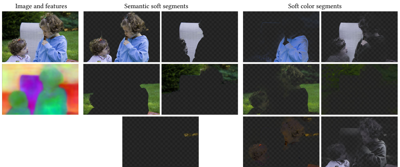
Fig. 13. Semantic soft segments by the proposed method and soft color segments by Aksoy et al. [2017b] shown together for conceptual comparison. Both methods are fully automated and only require the input image for soft segmentation.
