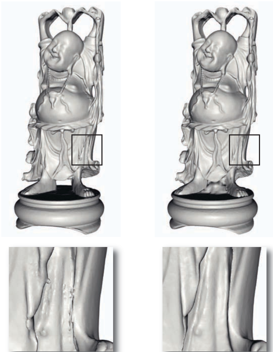
Figure 3.9: Reconstructions of the “Happy Buddha” model using VRIP (left) and Poisson reconstruction (right). Although our method generates a more accurate reconstruction of the sharp features, its independence of acquisition modality makes it incapable of leveraging line-of-sight information to carve out the space between the legs.
