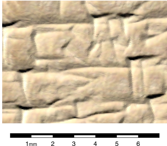
Figure 3. This enlargement from one of the tablet in our collection gives some indication of the current resolutions attainable with laser triangulation - ca. 50 micrometers, or 500 dpi. In a 2mm long wedge one can count approximately 40 data points; this yields about a 50 micrometers. We estimate our resolution requirement to be approximately 25 micrometers to capture all details.
