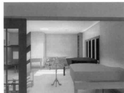
Plate 3: A particularly bad reference frame produced by our test-bed. Some areas of the image near the door were occluded in both reference frames, mostly because of prediction error.
