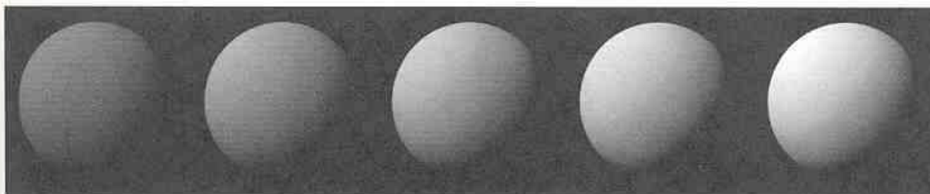
Fig. 16.3 Spheres shaded using a diffuse-reflection model (Eq. 16.4). For all spheres, I_p = 1.0 . From left to right, k_d = 0.4, 0.55, 0.7, 0.85, 1.0 . (By David Kurlander, Columbia University.)
