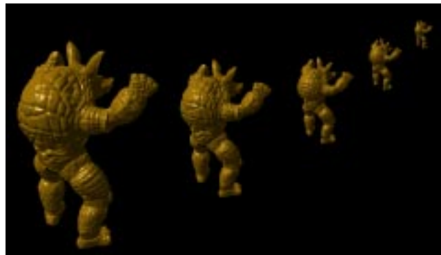
Figure 57: Levels of detail of the armadillo model shown with 1.0 mm maximum image deviation. Triangle counts are: 7,809, 3,905, 1,951, 975, 488
