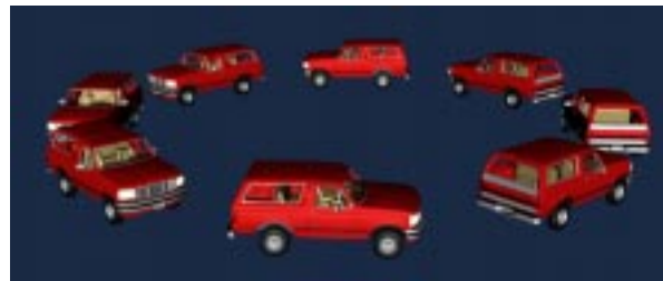
(b) 4 pixels (0.34 mm) of screen-space error: 94,000 triangles
