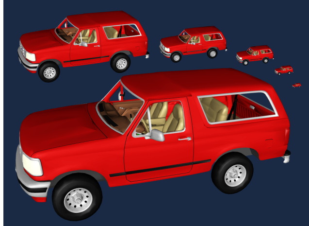
Figure 46: The Ford Bronco model at 6 levels of detail, all at 2 pixels of screen-space error (0.17mm)
