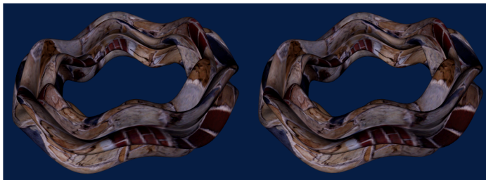
Plate 4: Wrinkled torus model at a transitional distance for 1 pixel of error (0.085 mm) 39,600 triangles 19,800 triangles
