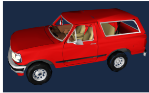
Plate 3: 26 pixels of error (4.4 mm) 9,000 triangles
